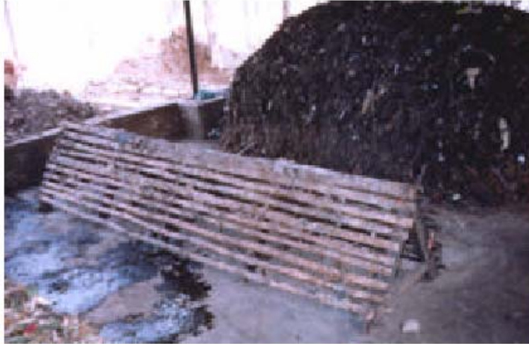
Figure 1.2: Bamboo frame for Indonesian windrow system in Dhaka, Bangladesh (Rytz, 2001)
